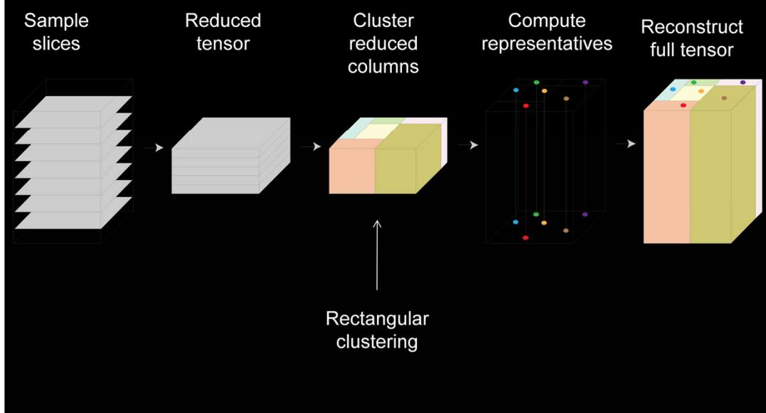
The extension will be done as follows: We compute a set of rows in every frame, resulting in a set of horizontal slices of the tensor.
