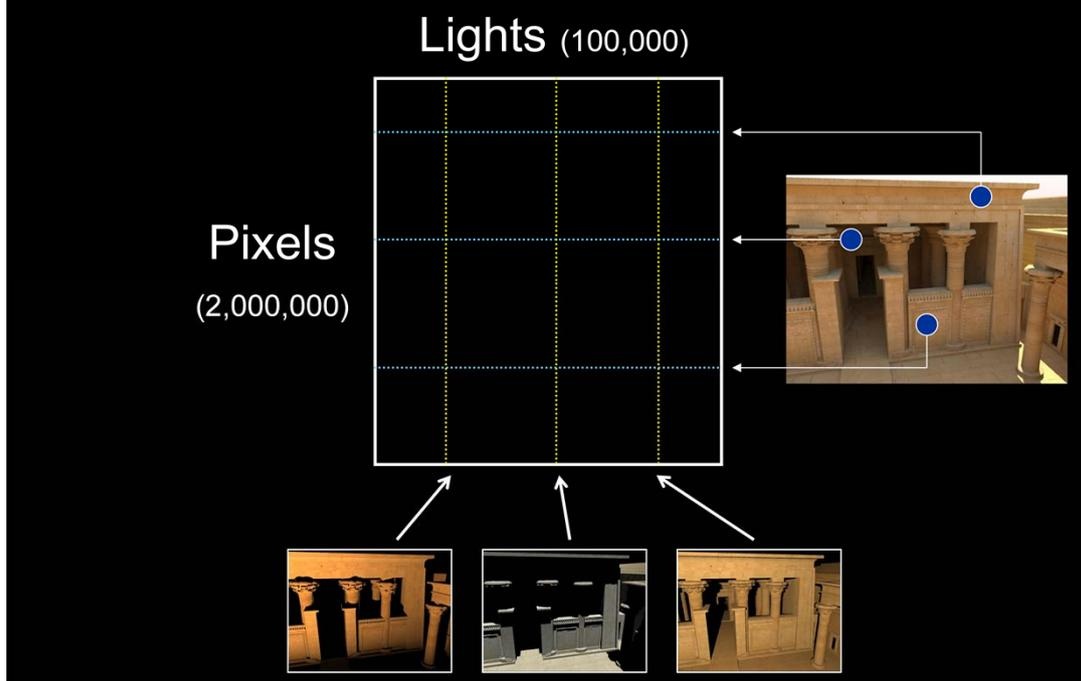
To get started in describing the algorithms, we first need to interpret the many light problem as a matrix of light-pixel interactions. This means that each element of the matrix is the contribution of a single light to a single pixel.
