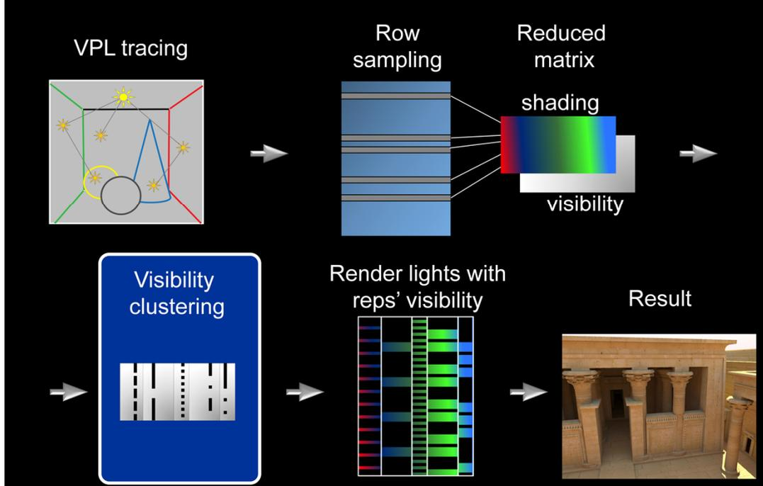
Here's the overview of visibility clustering. We start by distributing the global VPLs in the scene by tracing particles from light sources.
